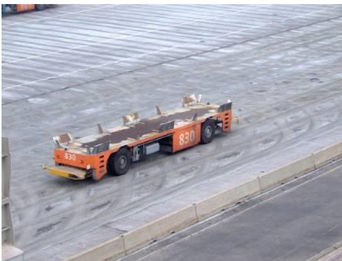
Fig 5: Automatic Container Transporter, Rotterdam Harbour
