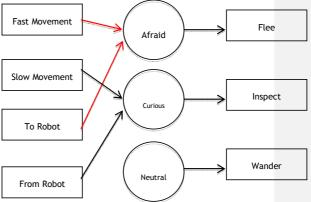
In these programs, it is important to make use of a State Diagram, which defines the states that a robot can adopt along with their associated actions. This is a further refinement of the Sense-Reason-Act loop.
