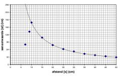
According to the graph, the value at 15 cm is about 120. Although the graph shows a maximum value of 250, the standard maximum is 1023. So: 120 / 1023 \* 100 = 12%
