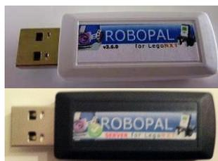
The special RoboPAL dongle uploads programs to the NXT via Bluetooth.
