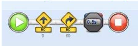
There is an icon that is not followed by a stopwatch so it will have a default waiting time of 1 sec. The robot will drive forward for 1 sec and then make a turn for 0.5 seconds.
