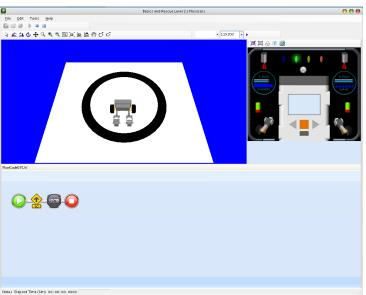
The simple program on the left shows you how to make a robot move forward for two seconds. You will make this program a little more interesting with each assignment. On the back of the instruction cards, you will find step-by-step instructions on how to develop and run this program. The idea is to make the robot stop at a black line.
