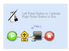
When the simulator starts, the CAL and RUN options will appear on the NXT screen. If you press the left button, the robot will start moving forward and memorising the values of the colours it meets. Please note that the calibration icon in the left top corner is needed to show the CAL and RUN menu.
