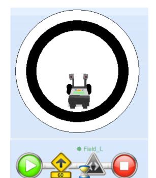
We can use this information to help the robot find out where it's going. This is much easier than having to count how long it takes to drive somewhere. Moreover, using a counter is not very accurate because when the batteries start running low, the robot will slow down. Also, if the robot starts out from a different place, things will often not work out as expected.
