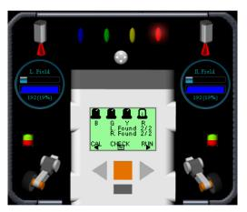
The robot can recognize colours, but you will need to tell it when to react to a colour every time. To do this you need to know about the change value of other colours. The sensors of every robot are all a little bit different, so you need to determine this value for every robot and every sensor. Not the best of situations.
